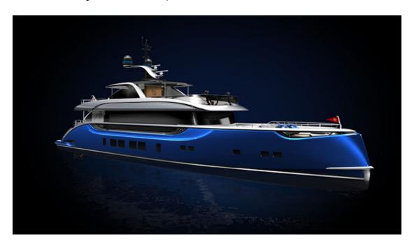
Each Dynamiq yacht should see top speeds around the low-20-knot range, with either MAN or MTU power and Fortjes pod drives. Van Oossanen's fast-displacement hull form should ensure more efficiency throughout the full speed range, too, thereby saving fuel and costs. As Dynamiq puts it, "The fast displacement hull can carry you from Monaco to Saint Tropez in just over 2 hours or make the trip from Miami to the Galapagos on one tank of fuel."
