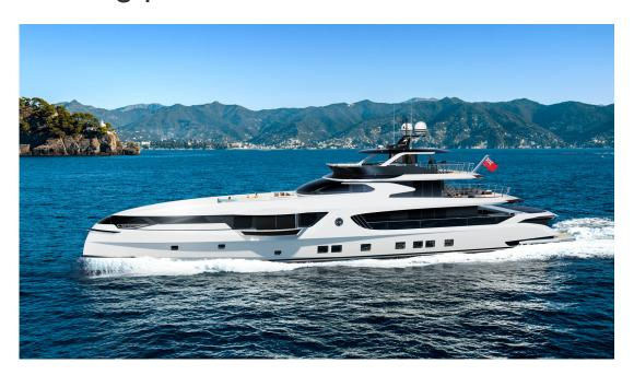
A hull vane and T-foil will provide lift when underway and hence reduce drag
