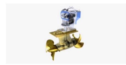
Aligned horizontally, Fortjes pods are supposedly much more efficient than any system using shafts and propellers. Their positioning outside the hull also means greatly reduced noise and vibration levels, as well as lower emissions. The pods use counter-rotating propellers linked via a compact gearbox to the main engines, reducing engine room space requirements by nearly 18%, which means more accommodation. Fortjes pods are built in Germany.
