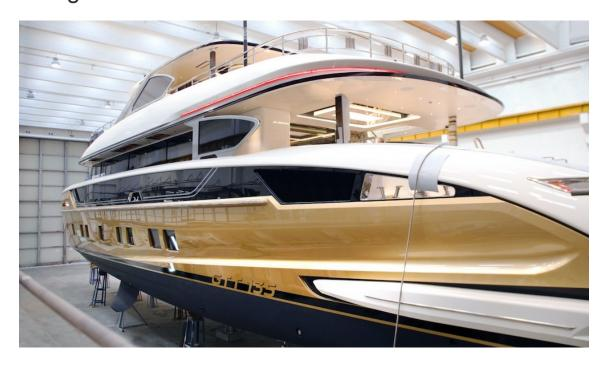
The hull of Dynamiq GTT 135 Stefania has a round-bilge shape for remarkably low resistance and low fuel consumption while still being capable of high speeds. The yacht is powered by twin MAN V12 1650 engines for a maximum speed of 20 knots with an ocean-going range of 3,500 miles at cruising speed. She has a shallow draft of 1.8 metres for cruising the remote cays and shoal waters of the Bahamas, for example.
