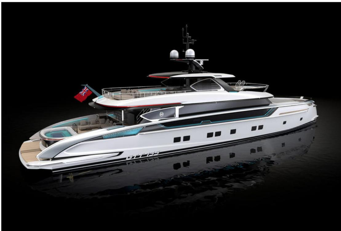
[Photo: Dynamiq Yachts](#) Featuring an exterior designed in-house, the *GTT 135* has been developed to slice through the water with ease. It has an optimal weight distribution and a low centre of gravity, which, when combined with the shape of the hull vane, give the yacht a 20% reduction in pitch and 30% reduction in hull resistance.
