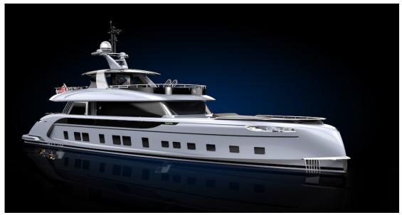
The GTT 115 features a round bilge aluminium hull and a specially engineered stabilisation system from Humphree with four electric fins and interceptors. The twin 1213kW MAN engines in conjunction with the latest Fortjes 5000 pods are able to propel the superyacht at a maximum speed of 21 knots. She is capable of crossing the Atlantic with a range of 3,400nm and with a shallow draft of just 1.45 metres (less than 5 feet), is perfect for the Mediterranean, Caribbean or Southeast Asia.
