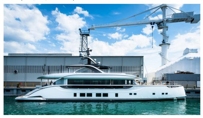
The two Dutch underwater specialists, Azure and Van Oossanen Naval Architects developed and optimised the slender and efficient hull on which *Jetsetter* is based. By fitting the yacht with twin Fortjes propulsion pods, *Jetsetter* offers a top speed of 21 knots with a cruising range of 3,000nm. To ensure a smooth experience while underway and at anchor, electrically driven CMC stabilisers are fitted to keep *Jetsetter* in shape no matter the conditions.
