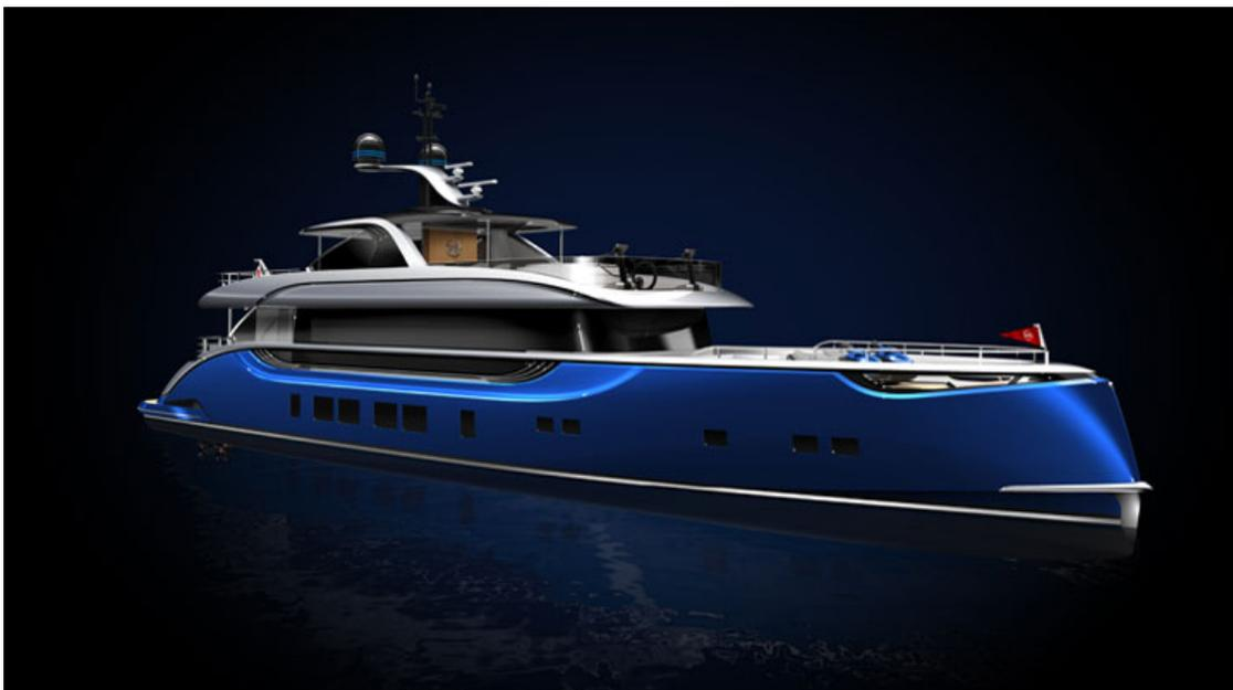
Each Dynamiq yacht should see top speeds around the low-20-knot range, with either MAN or MTU power and Fortjes pod drives. Van Oossanen's fast-displacement hull form should ensure more efficiency throughout the full speed range, too, thereby saving fuel and costs. As Dynamiq puts it, "The fast displacement hull can carry you from Monaco to Saint Tropez in just over 2 hours or make the trip from Miami to the Galapagos on one tank of fuel."
