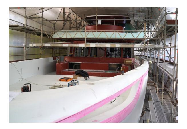
The D4 range was built as a fast family cruiser just below 40m, using a platform that designed with a shallow draught of only 1.7m.
